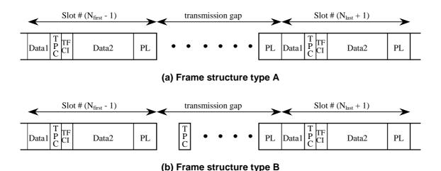
Figure 13: Frame structure types in downlink compressed transmission
